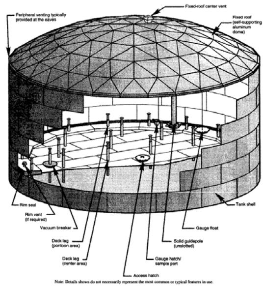
Figure 3. Covered Floating Roof Tank
