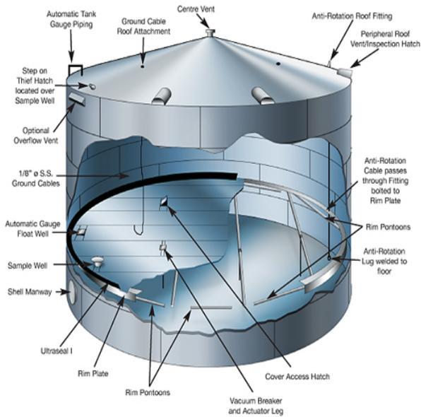
Figure 2. Internal Floating Roof Tank
