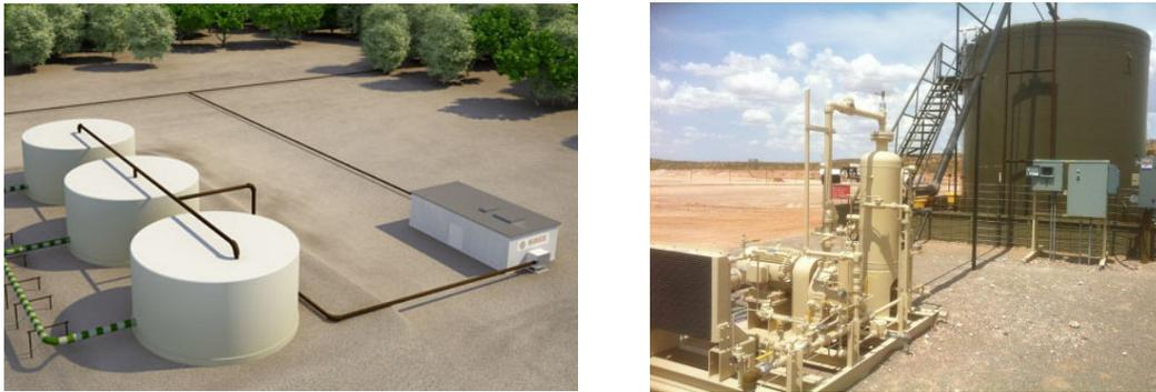
Figure 6. Vapor Recovery System
