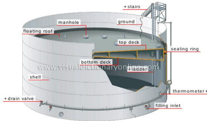
Figure 4. External Floating Roof Tank
