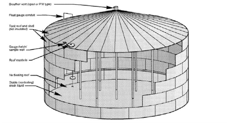
Figure 1. Typical Fixed Roof Tank
