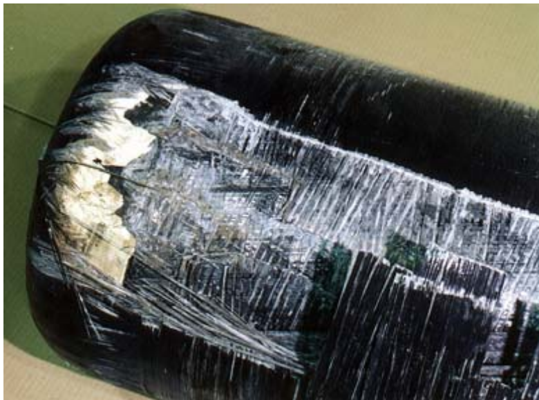
Figure 3 Type 3 cylinder damaged by bridge impact (from Newhouse et al.)
