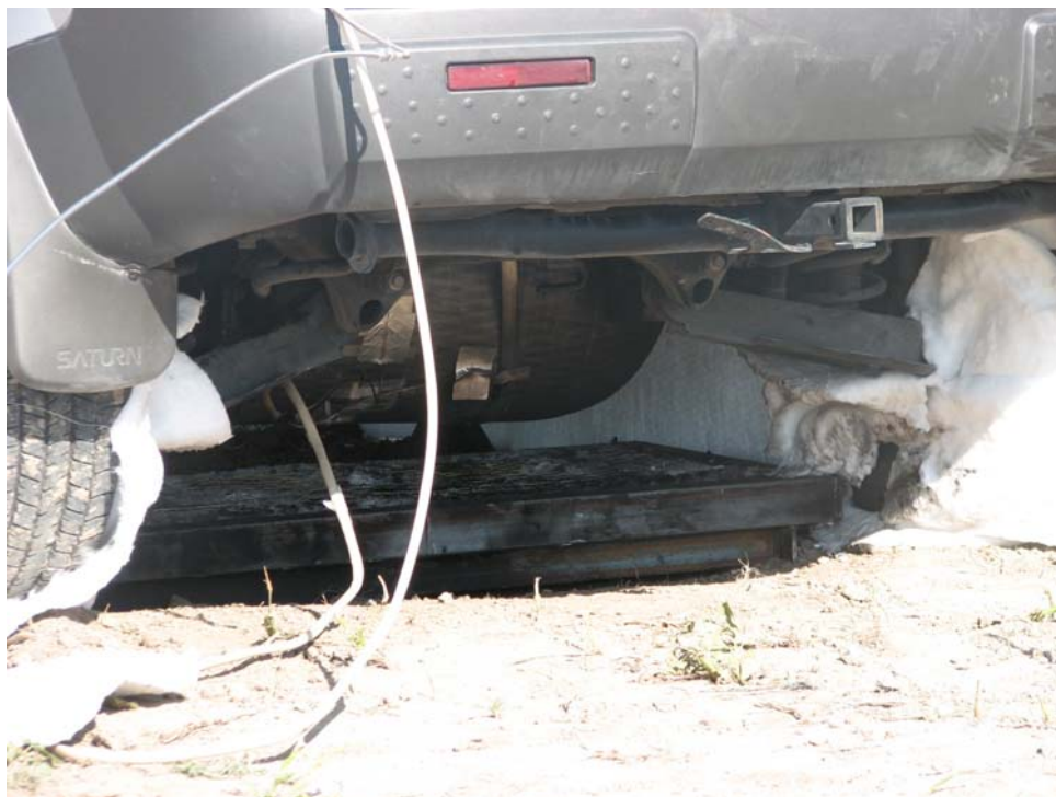
Figure 10 Burner below Type 4 cylinder under a SUV (from Zalosh)
