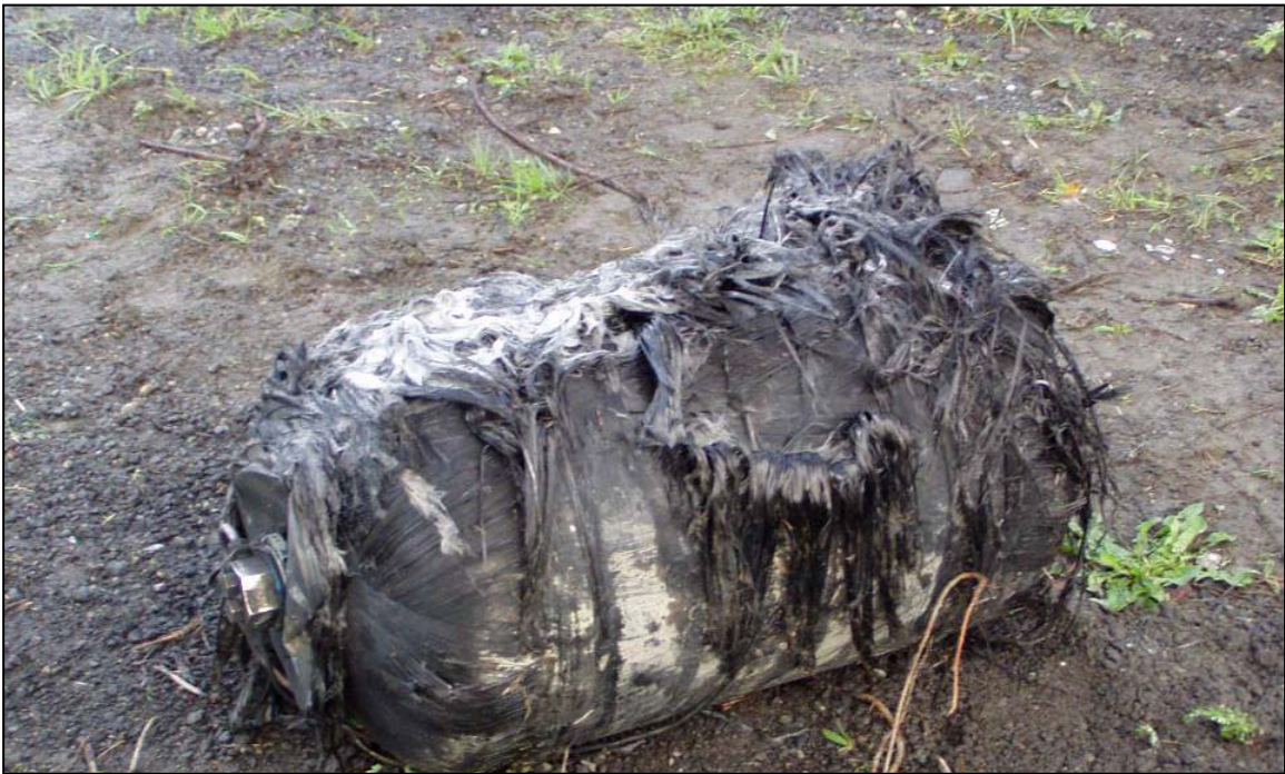
Figure 7. Ruptured cylinder remains from Honda Civic GX fire in Seattle.
