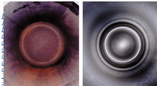
Figure 1. Internal photographs of cylinders in a) an "as-received" state and b) after surface treatment.
