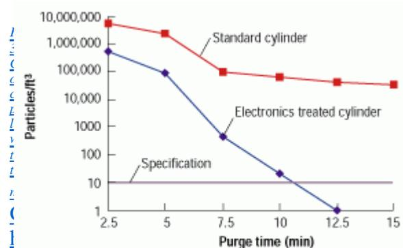
Figure 3. Comparison of cylinder particle levels with two treatment methods.
