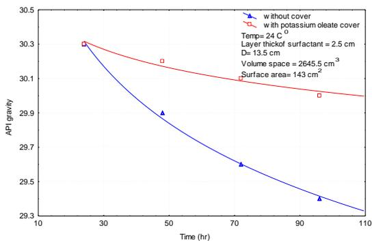
Fig. 21 API gravity vs. time.
