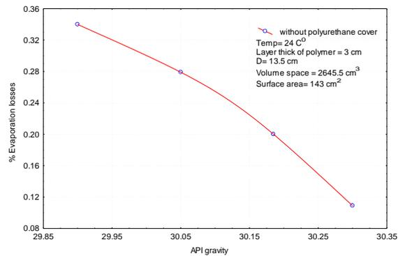
Fig. 23 percentage evaporation losses vs. API gravity with polyurethane cover.
