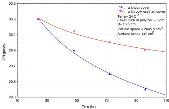
Fig. 20 API gravity vs. time.
