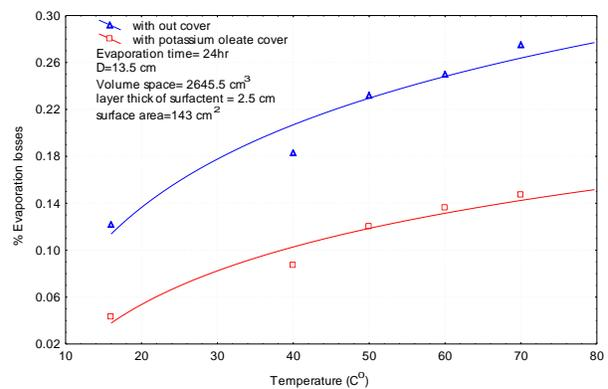
Fig. 6 percentage evaporation losses vs. temperature.
