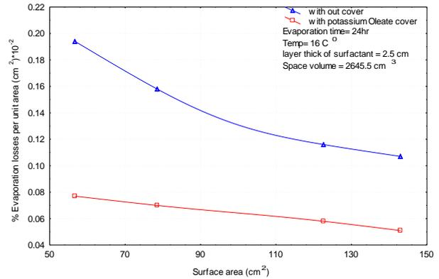
Fig. 10 percentage evaporation losses per unit area vs. exposed surface area.
