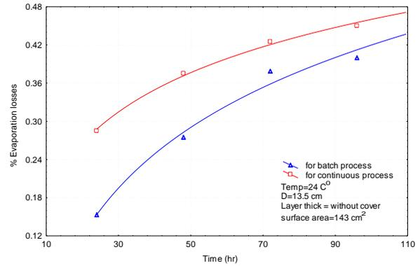
Fig. 17 compares between the evaporation losses of crude oil in the batch and continuous storage tank with out cover
