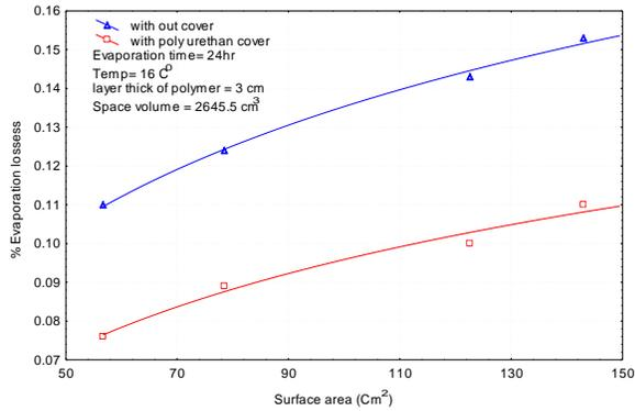
Fig. 7 percentage evaporation losses vs. exposed surface area.
