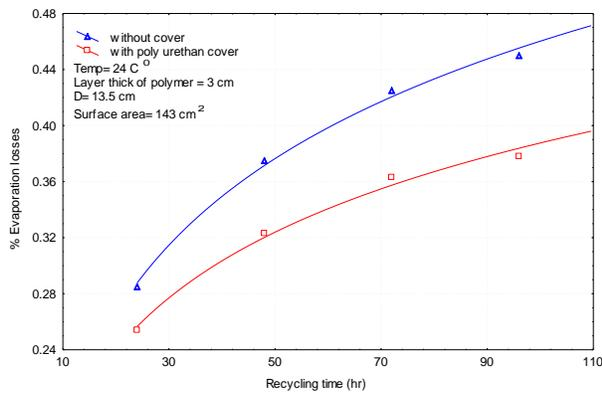
Fig. 15 percentage evaporation losses vs. recycling time.
