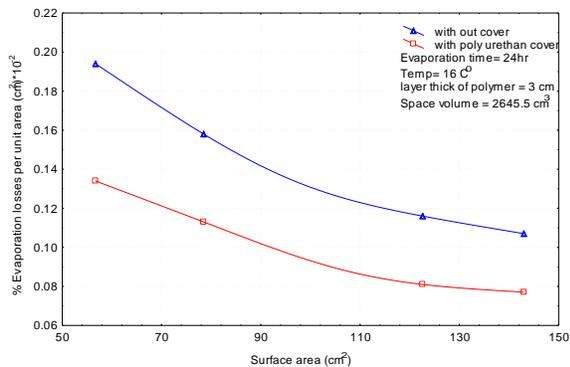
Fig. 9 percentage evaporation losses per Unit area vs. exposed surface area.
