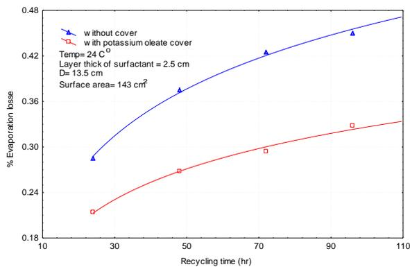
Fig. 16 percentage evaporation losses vs. recycling time.
