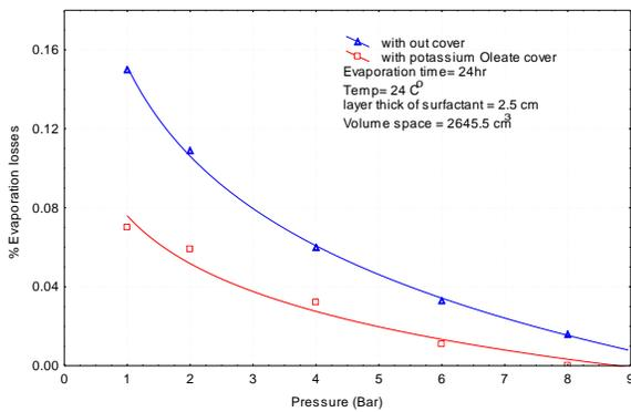
Fig. 12 percentage evaporation losses vs. pressure.
