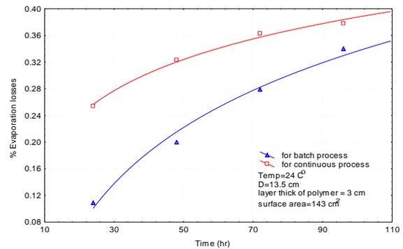
Fig. 18 compares between the evaporation losses of crude oil in the batch and continuous storage tank with polyurethane cover
