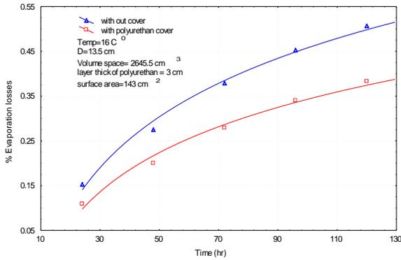
Fig. 3 percentage evaporation losses vs. time.
