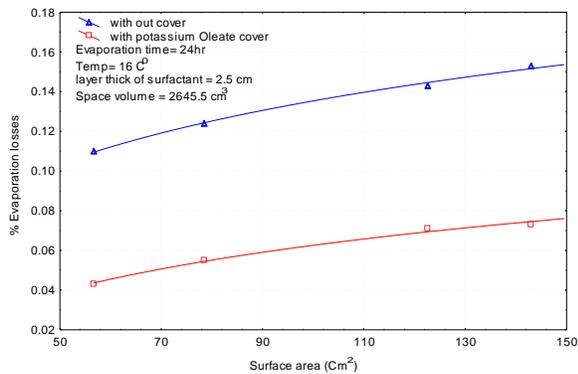
Fig. 8 percentage evaporation losses vs. exposed surface area.
