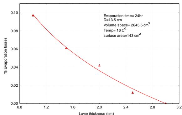
Fig. 1 percentage evaporation losses vs. Layer thickness with polyurethane cover.
