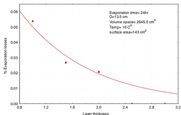
Fig. 2 percentage evaporation losses vs. Layer thickness with potassium oleate cover
