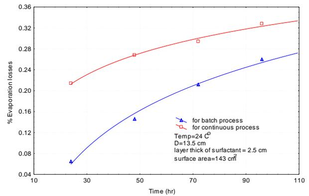
Fig. 19 compares between the evaporation losses of crude oil in the batch and continuous storage tank with potassium oleate cover
