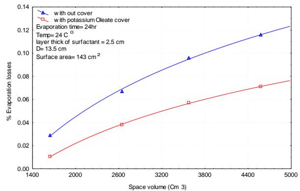
Fig. 14 percentage evaporation losses vs. space volume.
