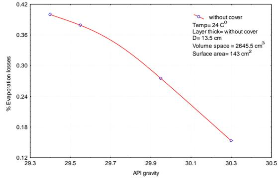
Fig. 22 percentage evaporation losses vs. API gravity with out cover.
