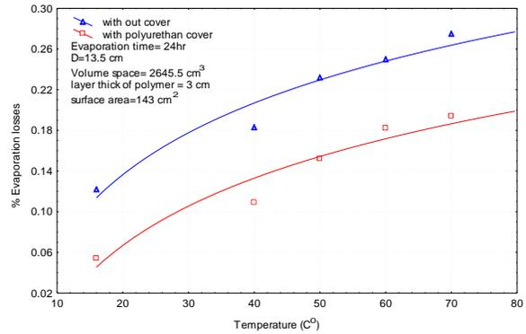
Fig. 5 percentage evaporation losses vs. temperature.
