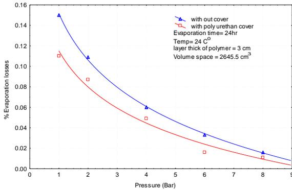
Fig. 11 percentage evaporation losses vs. pressure.
