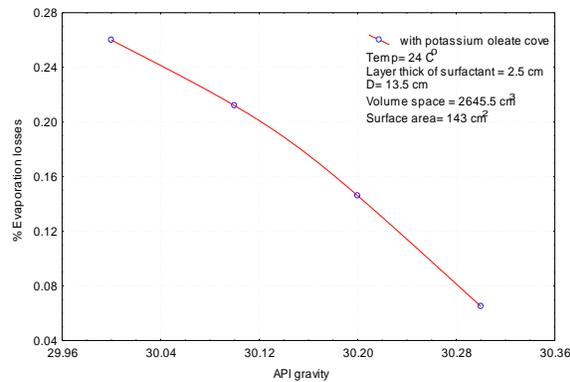
Fig. 24 percentage evaporation losses vs. API gravity with potassium oleate cover.
