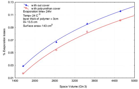
Fig. 13 percentage evaporation losses vs. space volume.
