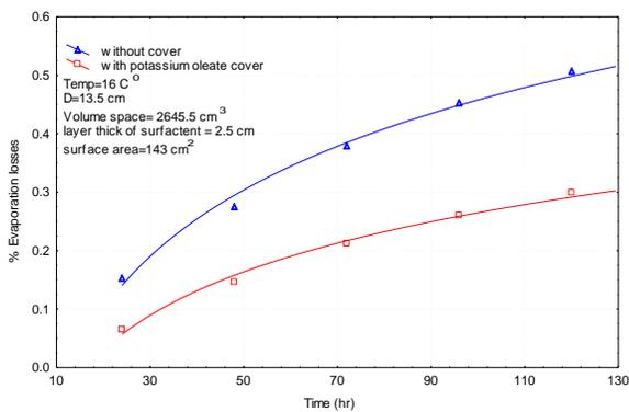
Fig. 4 percentage evaporation losses vs. time.
